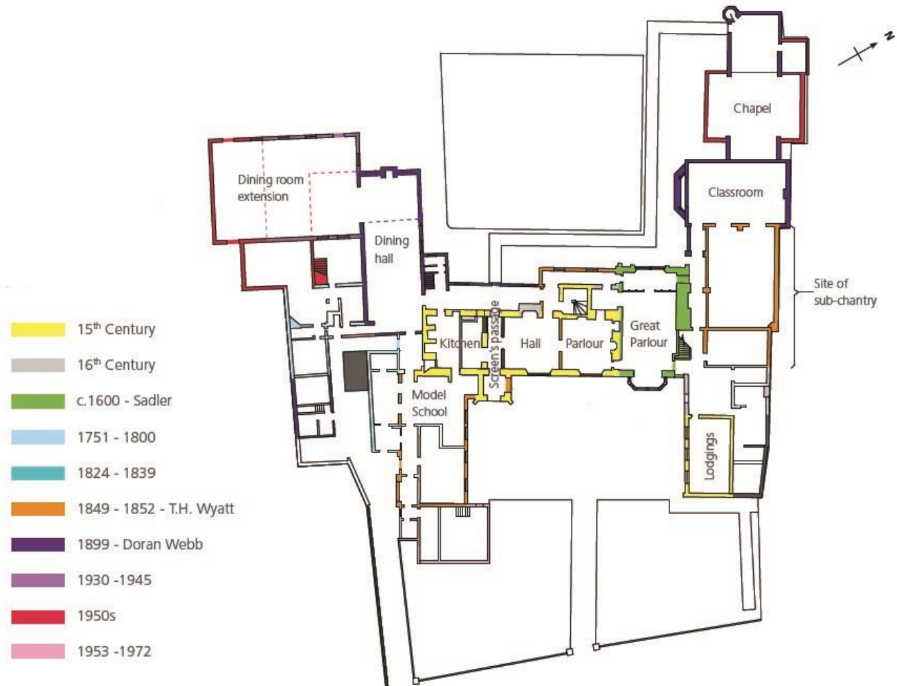
Ground floor plan of King's House showing different phases – plan drawn up in 2011 so does not reflect changes in 2014 and 2023
